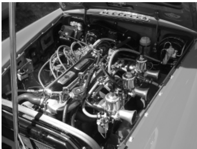
Photo Top Right: The GT was launched at the same time as the roadster. 2nd From Top: There was no “rubber bumper” version of the “C”. 3rd From Top: This restored car has non-standard Compomotive wheels. Lower Right: A Downton Stage 3 specification engine installed in the car illustrated above, with triple SU carbs and other tuning modifications.
